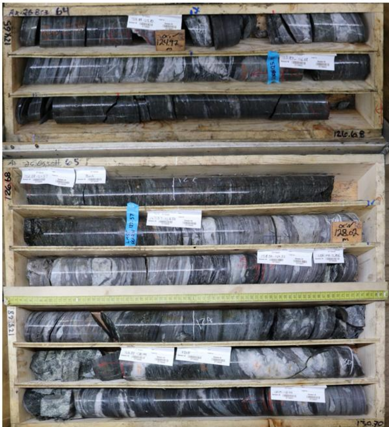
Figure 7: High-grade gold mineralization associated with replacement-style skarn mineralization. While sheeted quartz veins are the typical host for gold mineralization at Powerline, there is potential for mineralized skarn and calcareous metasedimentary units throughout Powerline and Airstrip.
