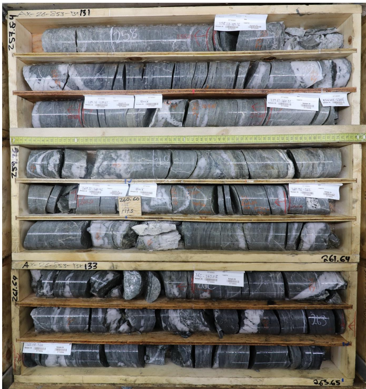
Figure 8: Mineralized sheeted quartz veins in Powerline, typical of intrusion-related gold systems and the majority of Powerline style mineralization.
