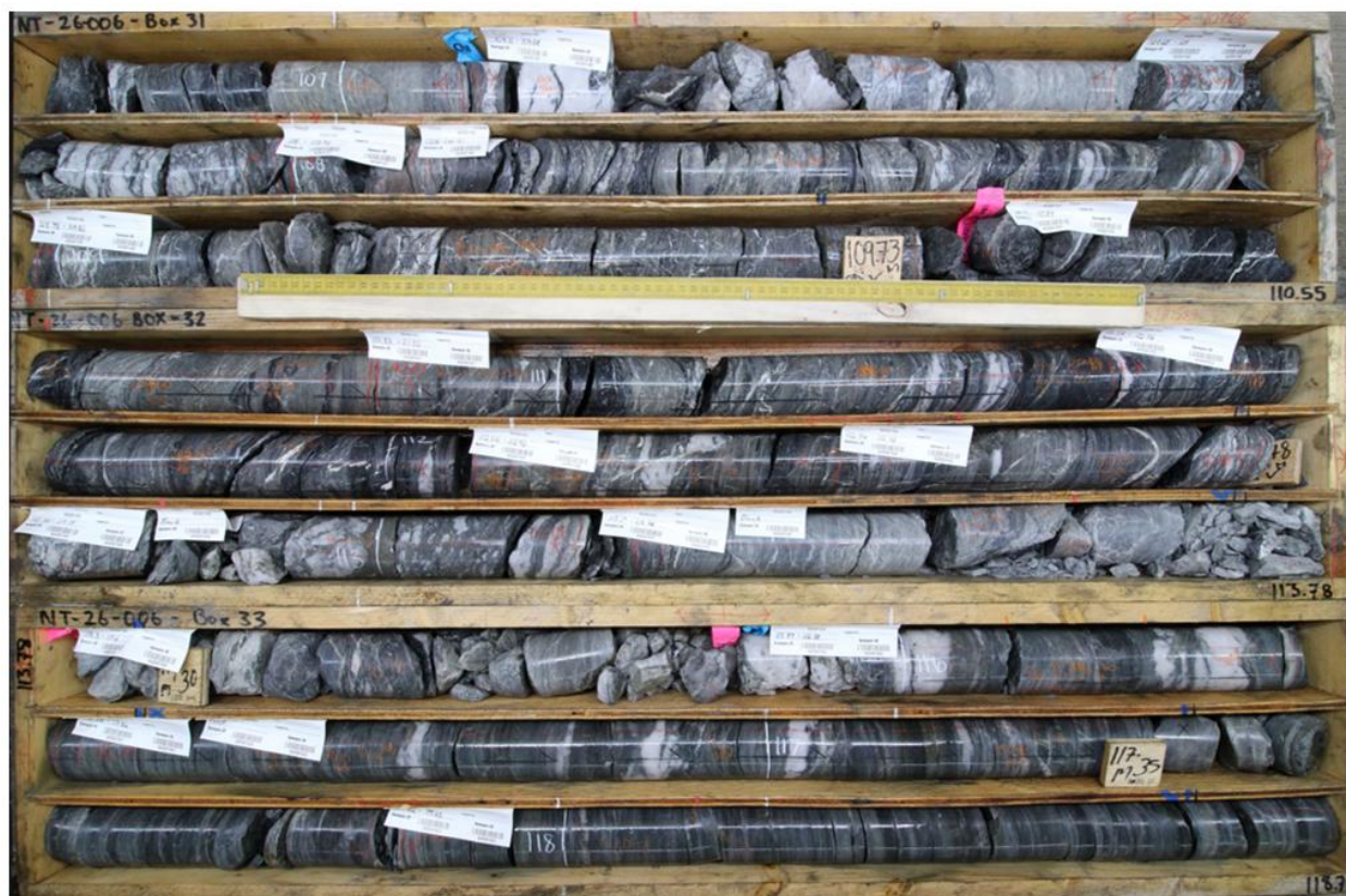
Figure 7: Zone of intensely sheared/deformed rock in drillhole NT-26-006 (Figure 3). Spatial association with visible gold mineralization from 36-53m in NT-26-006 is a strong indicator of potential for a more widespread mineralizing system at Seattle Creek.
