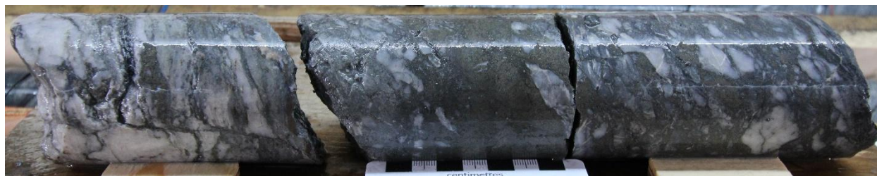
Figure 8: Brecciated quartz shear vein hosting bismuth sulphosalts, arsenopyrite, sphalerite, and pyrite. Late brecciation and mineralization of existing shear veins indicate a long-lived structure which underwent reactivation. Brecciation and mineralized ground mass may indicate high fluid flux through the system; reactivated structures may act as major fluid pathways for concentrating regionally pervasive mineralizing fluids.
