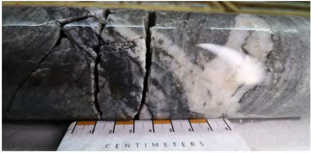
Extensional and shear quartz veins in NT-26-001. Top — 88.0 m, large extensional vein with bismuth-sulphosalts, sphalerite, arsenopyrite and pyrite (17.8 g/t Au over 87.9–88.3 m). Bottom left — 266.7 m. Bottom right — 162.9 m.
