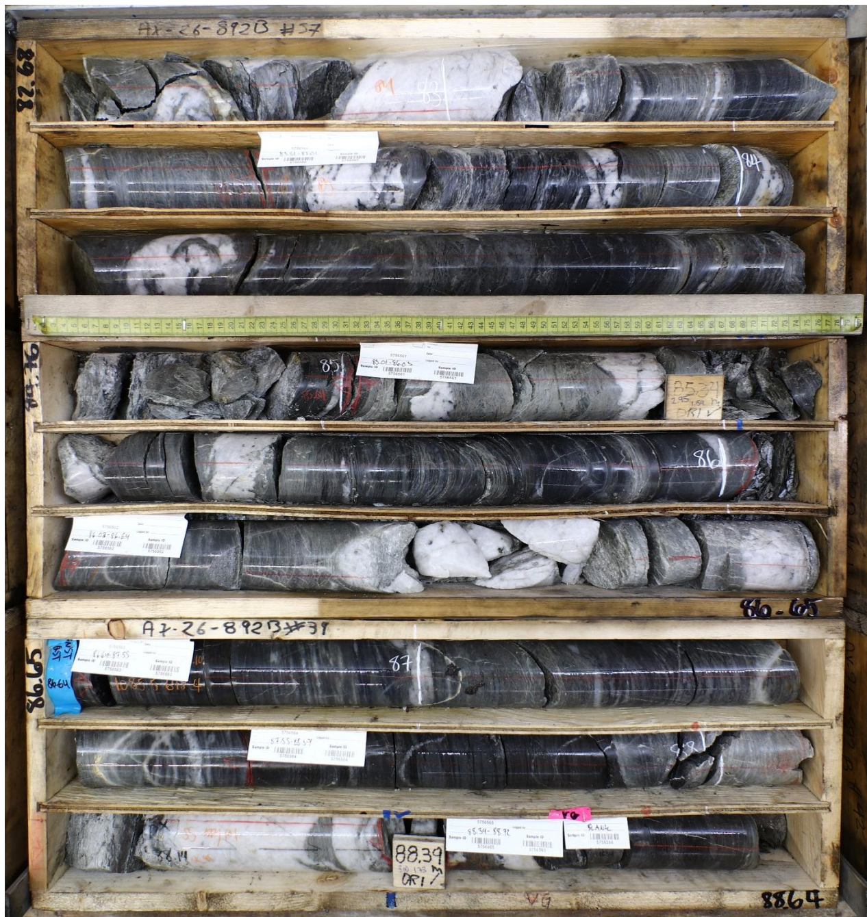
Figure 11: Mineralized extensional quartz veins in metasedimentary rocks in Powerline South from diamond drillhole AX-26-892B. High-density of large extensional quartz veins (>3 veins/m) with bismuth-sulphosalts, arsenopyrite, and pyrite are present throughout the interval from 87.6-140.4m, with multiple instances of visible gold (Figure 12).
